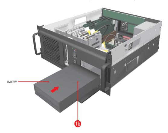
Figure 11. Inserting the New DVD-RW Drive
